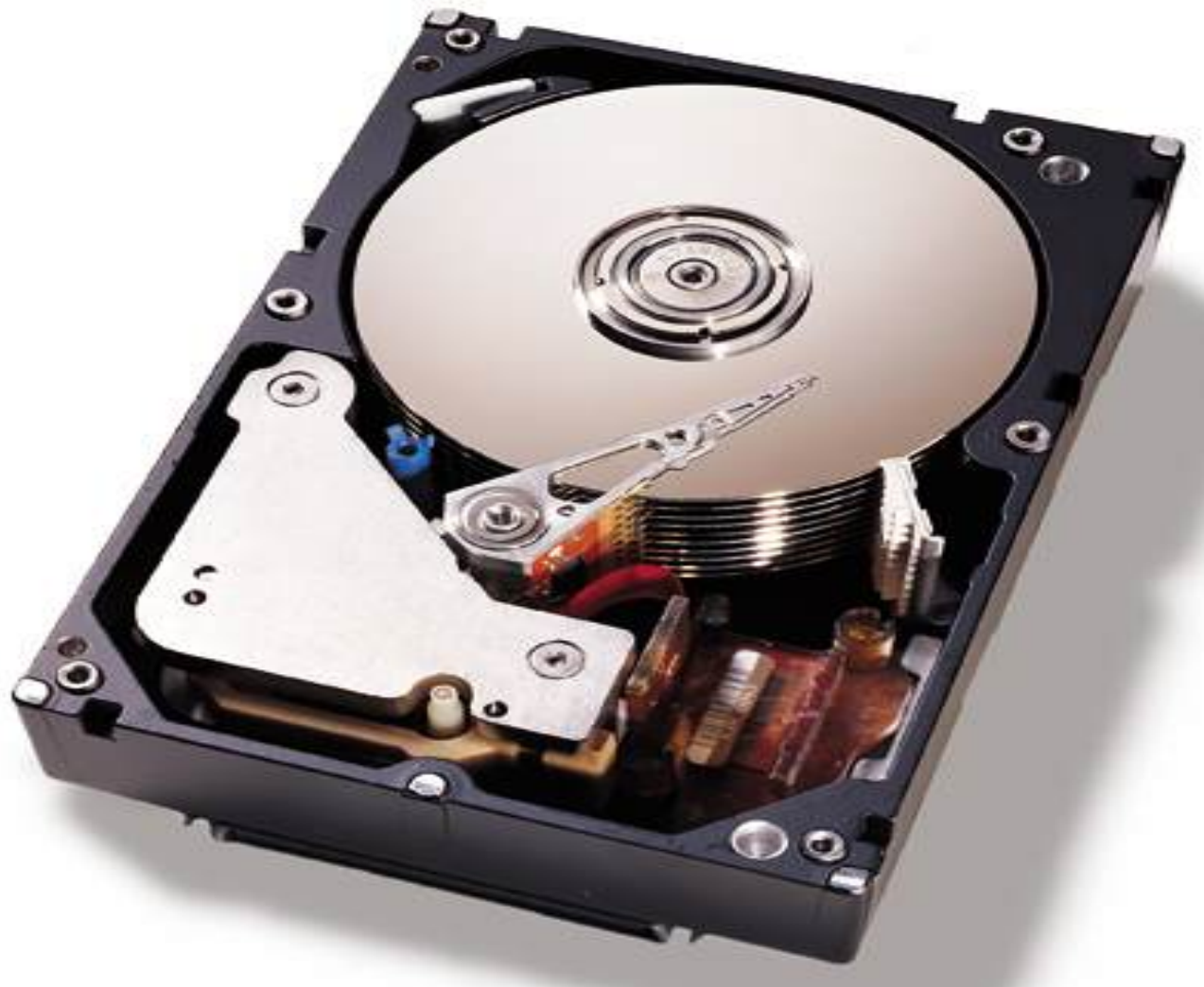
Top view of a 36 GB, 10,000 RPM, IBM SCSI server hard disk, with its top cover removed. Note the height of the drive and the 10 stacked platters. (The IBM Ultrastar 36ZX.)
